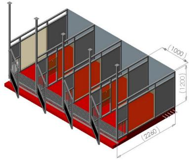
Example of Minipig pens with small area of slated floor in front. Suggested length and width is for a minimum size pen. They can be combined by a hatch for larger groups or built with a larger width. The height should not be lowered.
